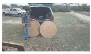
Cut two circles out of the 3/8 plywood not more than 39" in diameter – 39.00" seems to work OK, but will be "snug". If you want – make it a bit smaller and add foam into the gap to seal – path the foam black or use black foam.
