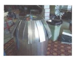
Secure the center of the inner eyelids to the 26" circle holes previously drilled. Secure with safety wire the center of the outer eyelids to the 26" circle in the center of the gapes life by the inner eyelids – should be about 1" or so. As you work your way around the circle you will have secured both inner and outer eyelids to the circle, forming a perfectly round shape and a much more stable structure.
