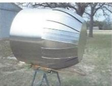
This time – we went back and pop riveted the outer eyelid corners to the inner eyelids using 1/8" pop rivets. It looks better and is more secure.
