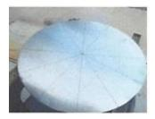
Cut a circle of aluminum 26: in diameter. Drill 1/16" or small enough for safety wire holes at 30 degree intervals at the end of the circle. This is to safety wire the inner eyelids to the circle to for the aft end of the AB.
